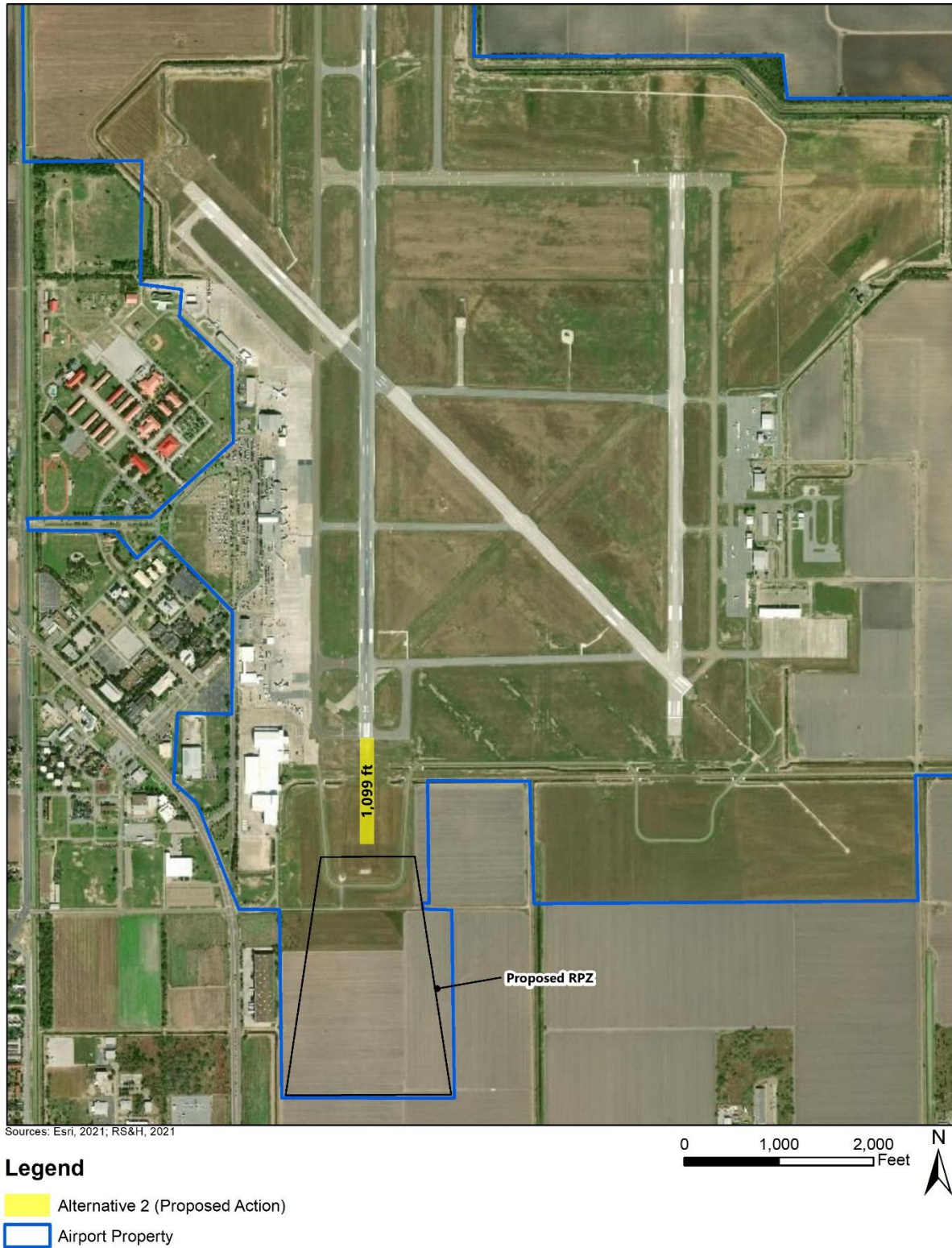
FIGURE 3-2 ALTERNATIVE 2: EXTEND RUNWAY 17R-35L 1,099 FEET TO THE SOUTH
